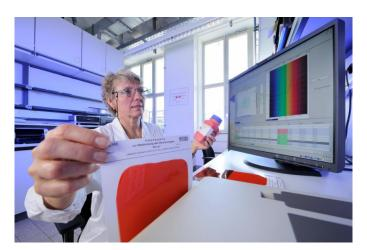
Remission measurement in a Leverkusen laboratory of the LANXESS Rhein Chemie business unit for quality control. Before the colorants are delivered to the customer, nuance (hue) and transparency of each production batch are determined and compared with the standard. The measurement is carried out on so-called test cards on which the color is applied. Photo: LANXESS AG
